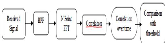
Input signal is passed through Band Pass Filter (BPF) of appropriate pass band to have a desired frequency band signal.
