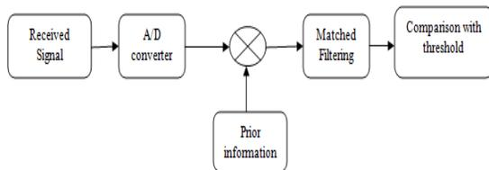
Input signal  $s(t)$  is passed through A/D converter to get discrete time signal  $s(n)$ . This signal further multiplied with prior information  $s^*(n)$ . [12]
