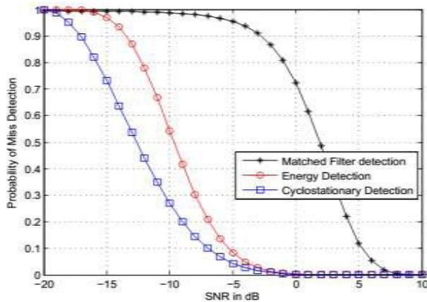
At -18 dB, cyclostationary detection is only scheme that can detect signal with low probability as in this scheme decision statistics is based upon noise rejection property of spectrum. Comparative analysis of three detection schemes in terms of  $P_f$ . Performance of energy detection scheme is worst in terms of  $P_f$  as it is a complete blind scheme i.e. it does not require any prior information.
